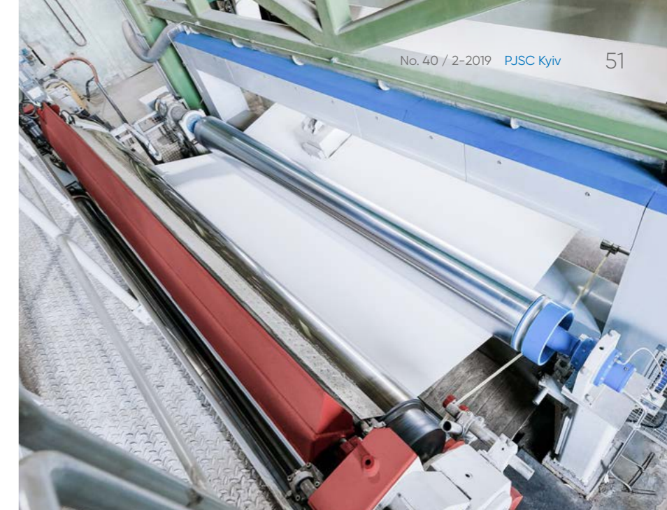
The new PrimeCal Hard hard-nip calender from ANDRITZ achieved the agreed smoothness parameters soon after start-up.
